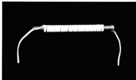
fig. 1. Loudspeaker lead can be formed into an rf choke by winding the lead around a ferrite antenna rod.
