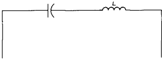
fig. 8. A practical capacitor has unavoidable inductance of leads as well as self inductance. At high frequencies inductance must be kept to an absolute minimum.
